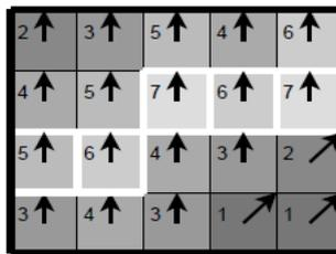
Fig. 3 Illustration of Non-maximum suppression.
