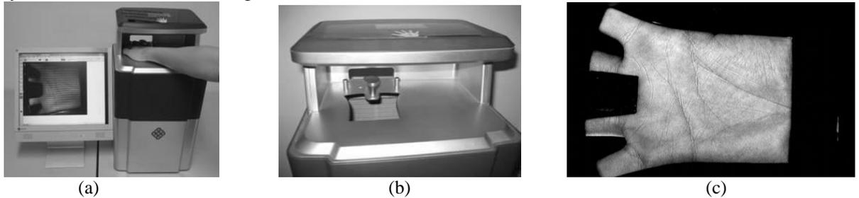
Fig.1. (a) the outlook of image acquisition device; (b) The device is being used to collect palm print image; (c) The “PolyU\_001\_F\_01.bmp” palm print image. [6]
