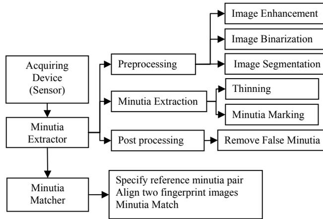
Fig.2. Fingerprint Recognition System
