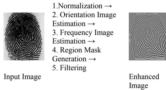
Fig.5. Flowchart for fingerprint enhancement algorithm
