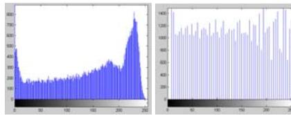
Fig.3. (x) before histogram equalization (y) after histogram equalization.
